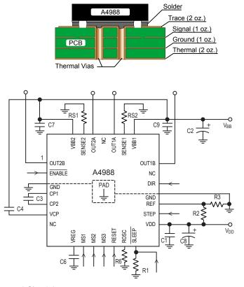
Figure 8: Typical Application and Circuit Layout
