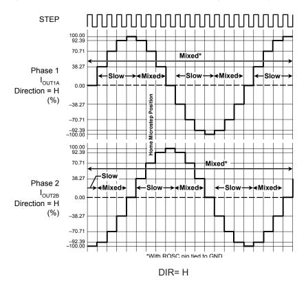
Figure 11: Decay Modes for Quarter-Step Increments
